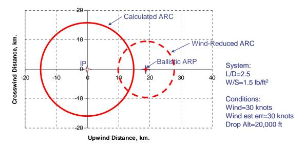
The next example is for a low-glide system with low wind uncertainty, typical of using a dropsonde within 10 minutes of release. The raw release circle is much smaller than the mid-glide system and good wind data is needed to maximize the wind-reduced release circle. The usable air release circle would take approximately 120 seconds to traverse at 120 knots.
