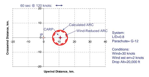
Now consider a high-velocity (160 f/s) two-stage system with low L/D using "aged" winds with high uncertainty. The flight planner could choose to ignore the forecast and drop directly over the IP and still have a successful delivery. Note the change of scale. Both the circle sizes and the ballistic offset are reduced because of the high vertical velocity. The additional landing dispersion during unguided final descent is not included in the diagram.
