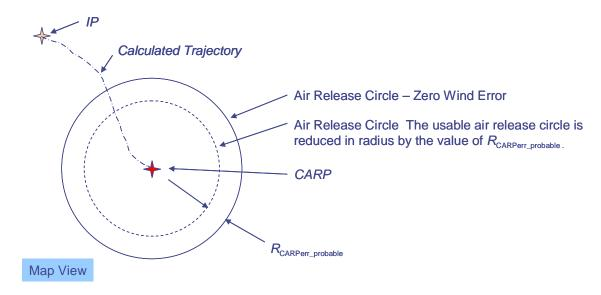
A few examples are useful to illustrate how the effects of wind, wind uncertainty, glide ratio, and true airspeed are combined in an ARC diagram. The first example is for a mid-glide system descending 20,000 feet through a mean wind of 30 knots with an uncertainty of 10 knots. One-third of the available offset is needed to overcome wind uncertainty.
