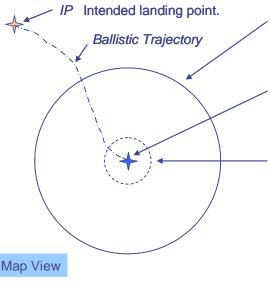
Air Release Circle With zero wind error, a system released inside this circle is capable of reaching the IP.
