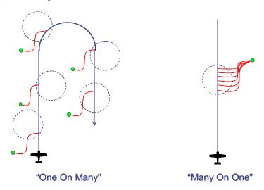
In each diagram the aircraft flies into a calculated air release circle, shown as dashed circles, releases one or more cargo units within that circle in order to deliver to the IPs, shown as small circles.
