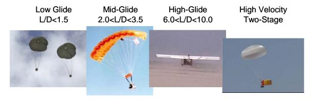
Low-glide types include controlled conventional cargo parachutes and single-surface gliding type parachutes. At this time only the former is represented.
